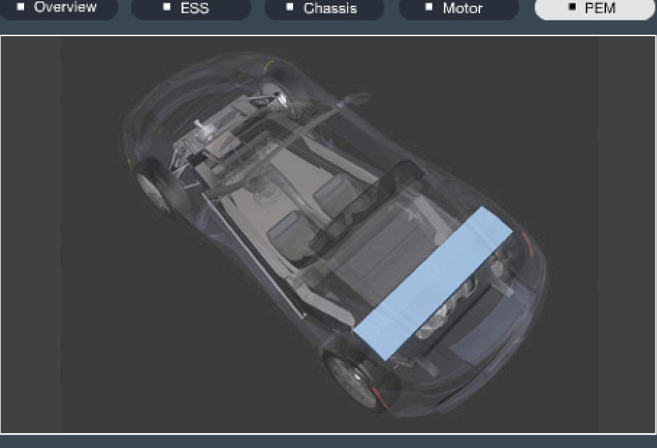
The Power Electronics Module (PEM) contains high voltage electronics that control the motor and allow for integrated battery charging. The motor and PEM have been designed as a tightly integrated system that delivers up to 185 kW of motor output.
