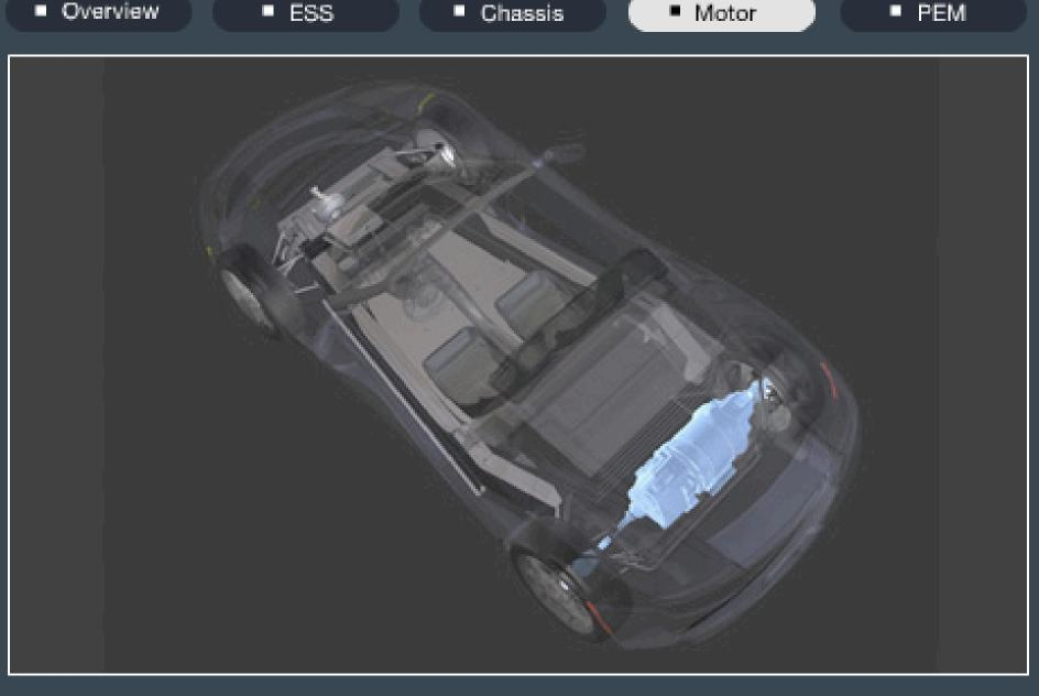
The Tesla motor weighs less than 70 pounds yet produces horsepower equivalent to a much heavier internal combustion engine. And unlike a gasoline engine, Tesla's electric motor doesn't sacrifice mileage for performance.
