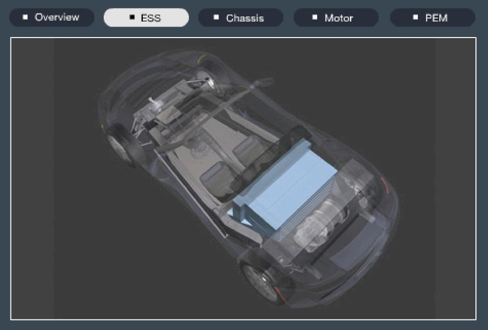
The Energy Storage System (ESS) – comprised of several thousand consumer-grade lithium-ion cells – is the heart of the Tesla Roadster. Battery conditions are continuously monitored and fed to the Vehicle Management System (VMS), allowing for precise tracking of battery history, performance, and available energy.
